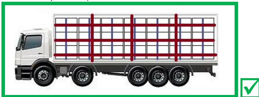
Diagram 4 – correct protection of waste paper bales with belts and rack elements (Protection of the bales is marked by blue colour).
