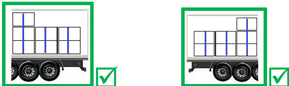
Diagram 9 – an example of waste paper bales loaded compatibly with work safety and hygiene rules - one row directly by three rows, protected with belts (Protection of the bales is marked by blue colour).
